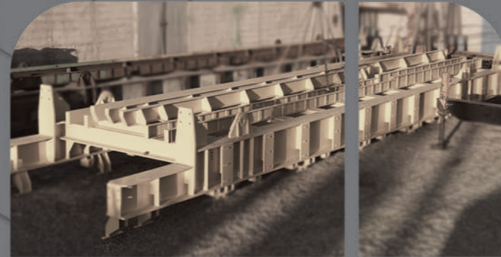
Apron Feeder Framework
