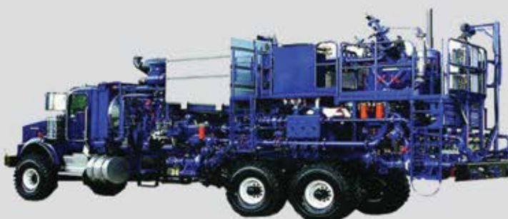
Truck mounted cementing unit
